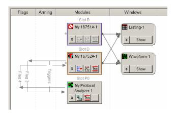
Note that the trigger icon and menu items are enabled — this shows the connection is active and lets you change the cross-triggering or trigger deskew setup.
